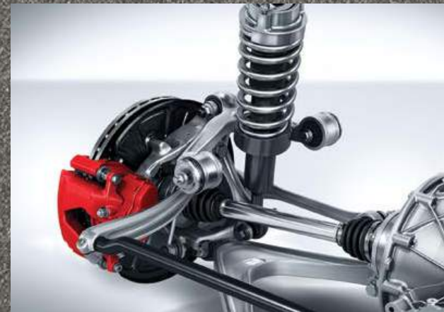
AMG high-performance composite brake system with red brake callipers.
