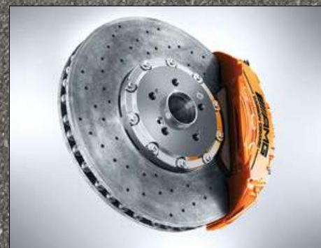
AMG high performance ceramic composite braking system
